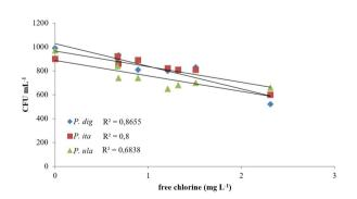
**Figure 4.** Correlation between free chlorine of acidic water produced by PE-1 machine and count of 3 pathogen species; *P. digitatum, P. italicum* and *P. ulaiense*. Regression coefficient represented by R<sup>2</sup> value.
