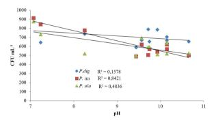
**Figure 3.** Correlation between pH of alkaline water produced by PE-1 machine and count of the 3 pathogen species; *P. digitatum, P. italicum* and *P. ulaiense*. Regression coefficient represented by R<sup>2</sup> value.
