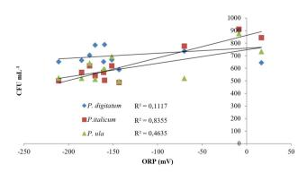
**Figure 2.** Correlation between ORP of alkaline water produced by PE-1 machine and count of 3 pathogen species; *P. digitatum, P. italicum* and *P. ulaiense*. Regression coefficient represented by R<sup>2</sup> value.
