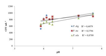
**Figure 6.** Correlation between pH of acidic water produced by PE-1 machine and count of 3 pathogen species; *P. digitatum, P. italicum* and *P. ulaiense.* Regression coefficient represented by R<sup>2</sup> value.
